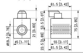
With coils having bi-directional diode and bipolar sheathed free lead, 350 mm long, without pins.
