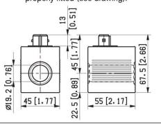
With coils having bi-directional diode and bipolar sheathed free lead, 350 mm long, without pins.
