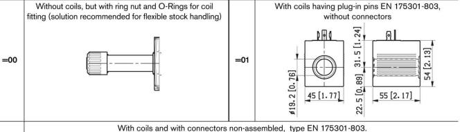
Protection class: IP 65 when connector with seal is properly screwed down, and cable clamp is correctly tightened.
