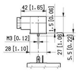
With coils having AMP Junior connector, and with bi-directional diode.
